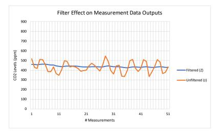
The graph above shows the effects of the filter on the CO<sub>2</sub> measurement data (Z or z). The unfiltered output is shown in orange and the filtered output shown in blue.
